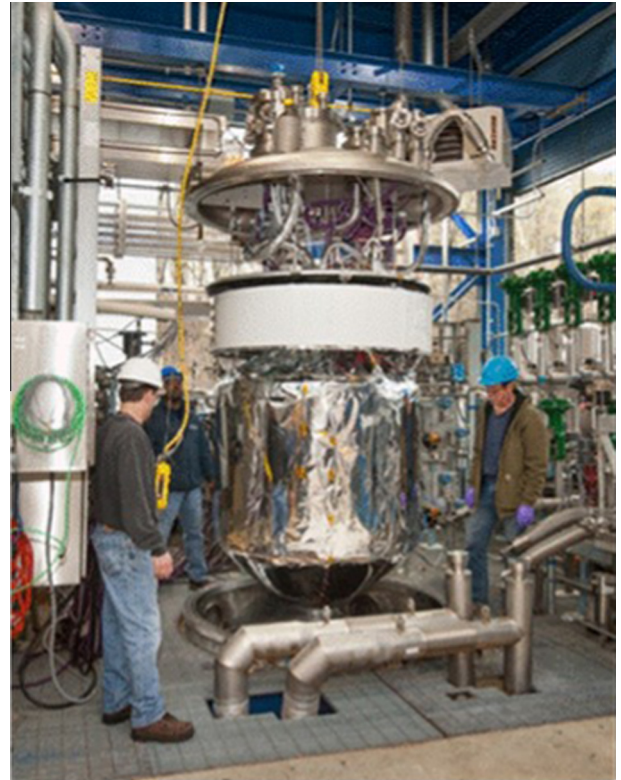
Fig. 1. \text{LO}_2 ZBO test article being lowered into the vacuum chamber.
